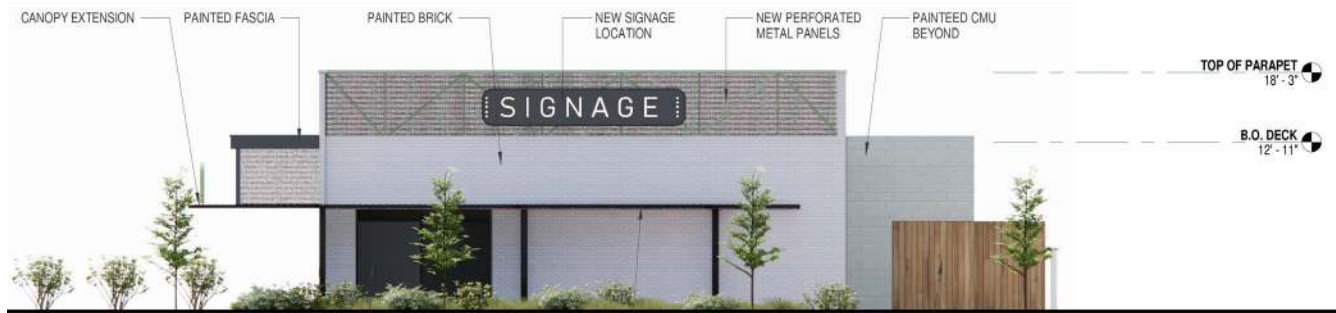
PROPOSED ELEVATION - SOUTH SCALE: 1/8" = 1'-0"
